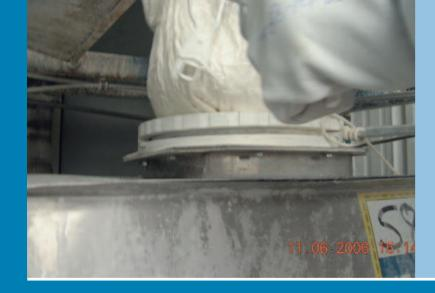
Secure the bag to the Hopper to prevent spillage.
